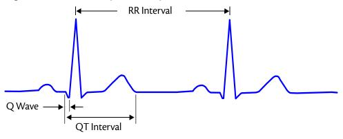
Figure 4.15 illustrates the Q wave, QT interval and the R-R interval. A normal QT interval should be less than half the R-R interval. A prolonged QT interval is associated with increased risk of R-on-T triggered lethal dysrhythmias.
