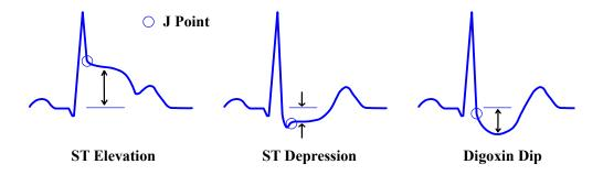
Figure 4.17 presents three examples of ST deviation. A digoxin dip is also called a "dig dip".
