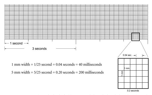
Figure 4.8 provides details of ECG paper. Note the larger hash marks that indicate 3 second intervals. Two 3 seconds intervals (6 seconds) is often used to determine heart rate.
