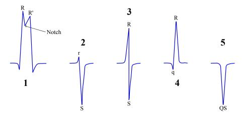
Figure 4.14 depicts several QRS complex shapes or morphologies. QRS complex #1 demonstrates the labelling convention for subsequent positive deflections above the baseline after the R wave. This second deflection is labelled R'. Note that a third upright deflection would be labelled R''(R double prime). QRS complex #2-4 are all normal QRS complexes of different shapes. QRS complex #3 is a biphasic QRS complex would be labelled RS. The QRS complex #5 is a OS complex.
